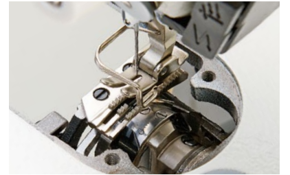
Upper side of the thread-trimming knife
